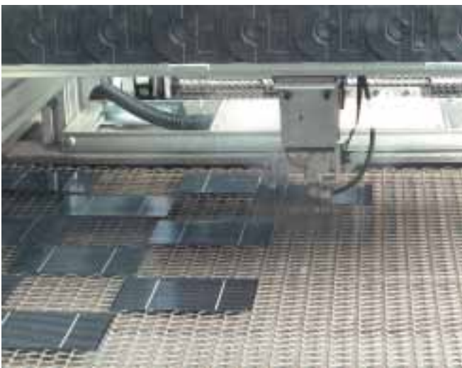
Custom-built robots perform most of the handling of the delicate silicon cells.
