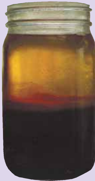
As the test batch settles, two layers appear: biodiesel fuel on top and glycerin on the bottom.
