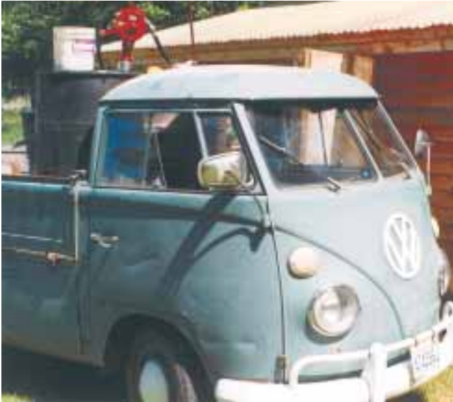
Scott's used veggie oil collection rig with barrel and pump.
