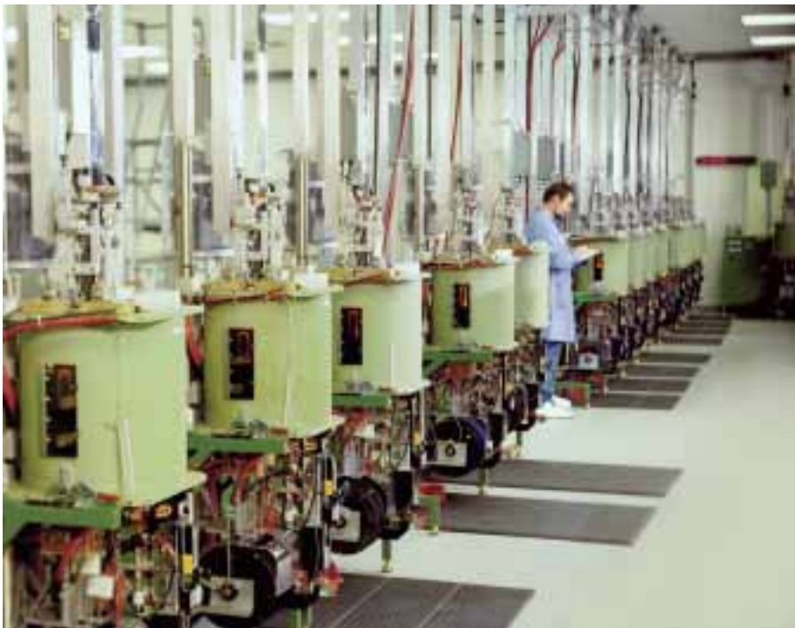
A line of String Ribbon silicon furnaces produce tomorrow's photovoltaic cells.
